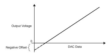
When the output amplifier has a positive offset, a digital input of zero does not result in a zero output voltage. The DAC12 output voltage reaches the maximum output level before the DAC12 data reaches the maximum code. This is shown in Figure 19–5.
